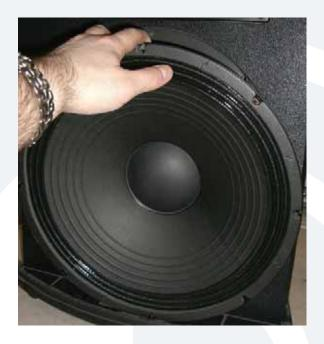
Carefully begin to remove the woofer. This woofer has a tendency to want to pop out, so please be sure to hold the woofer in place with your free hand while removing the screws with the other
